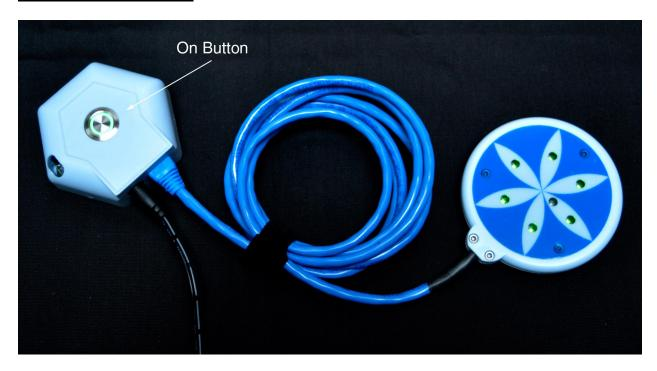
After programming the device, unplug the USB cable from the top of the MR71. Next, push the On/Off button on top of the device. The MR71 is on when there is green ring around the button. When on, the Magnetic Disk LEDs will flash.
