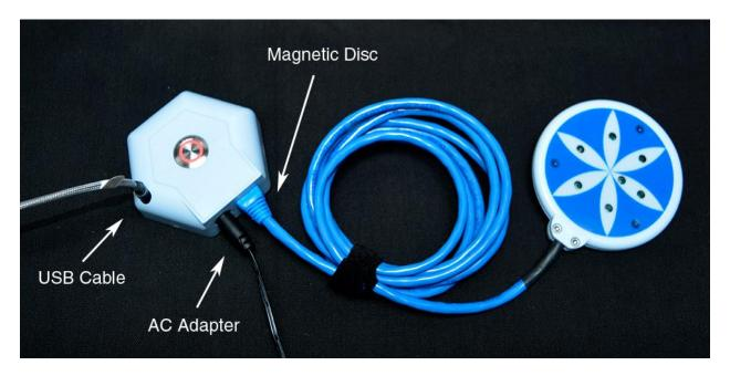
Insert the round end of the AC Adapter cable into the round port of the **MR71** (as shown above). Plug the other end into a 120 volt electrical outlet. The **MR71** must be plugged in order for it to be programmed or to operate. Also, make sure the **MR71** is Off. The On/Off button is located on top of the device in the middle. The unit is On when the button has a red ring around it.
